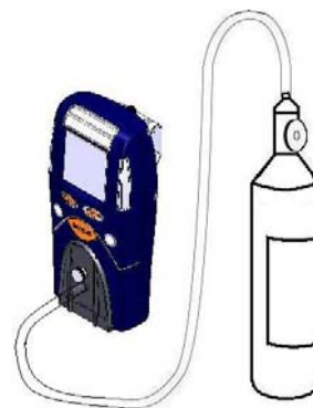
Figure 4.1 Bump Test / Gas calibration set up
